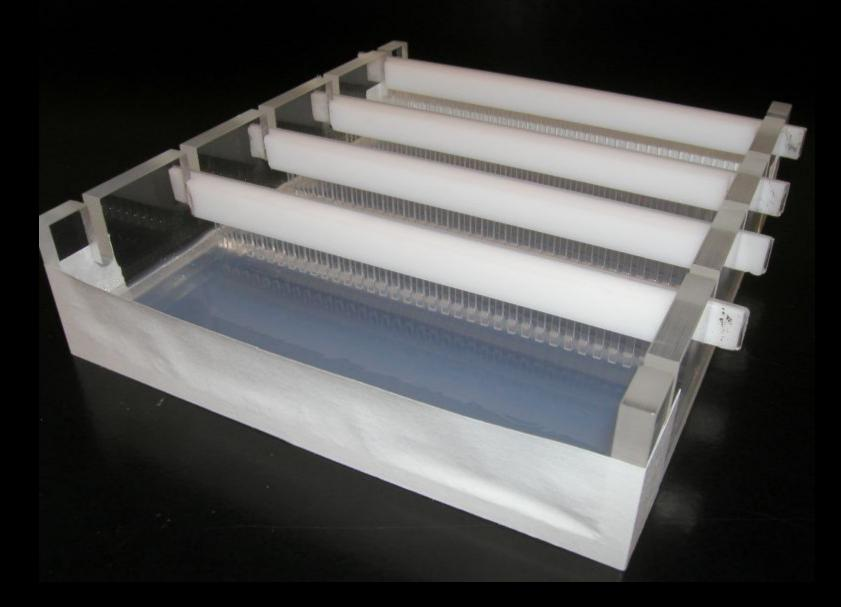
When cooled, the agarose polymerizes, forming a flexible gel. It should appear lighter in color when completely cooled (30-45 minutes). Carefully remove the combs and tape.
