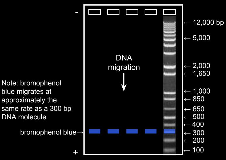
Inclusion of a DNA ladder (DNAs of know sizes) on the gel makes it easy to determine the sizes of unknown DNAs.
