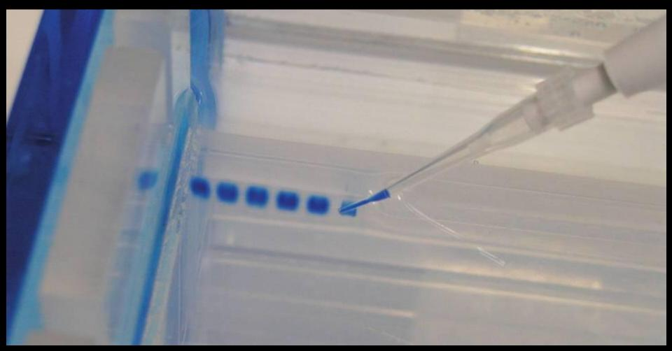
Carefully place the pipette tip over a well and gently expel the sample. The sample should sink into the well. Be careful not to puncture the gel with the pipette tip.
