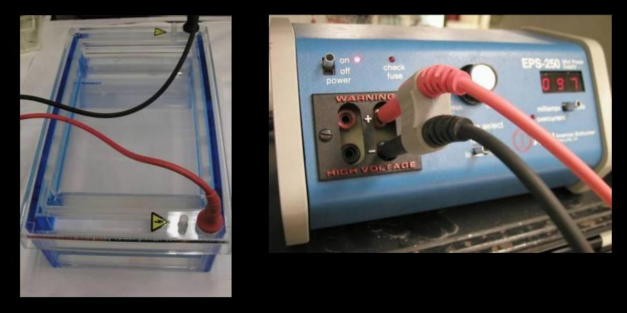
Place the cover on the electrophoresis chamber, connecting the electrical leads. Connect the electrical leads to the power supply. Be sure the leads are attached correctly - DNA migrates toward the anode (red). When the power is turned on, bubbles should form on the electrodes in the electrophoresis chamber.
