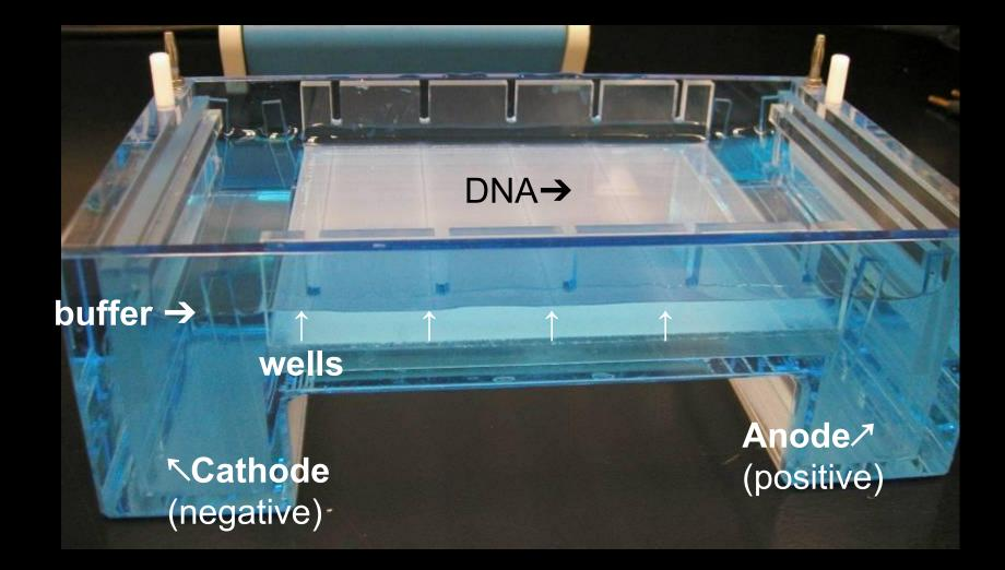
Add enough electrophoresis buffer to cover the gel to a depth of at least 1 mm. Make sure each well is filled with buffer.
