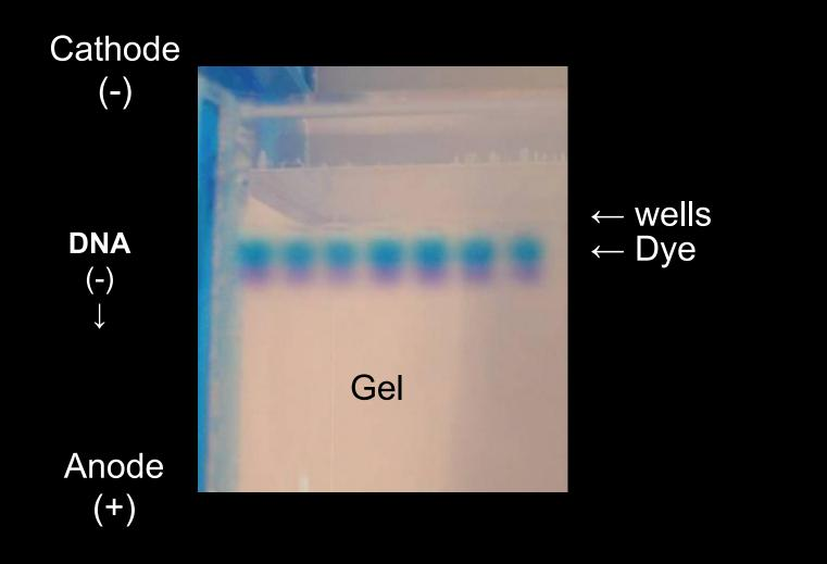
After the current is applied, make sure the Gel is running in the correct direction. Dye will run in the same direction as the DNA.
